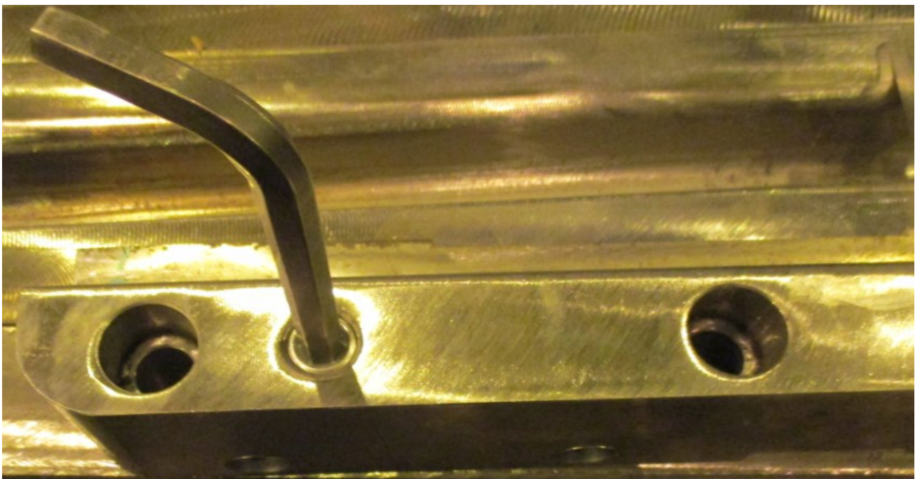
Loosen the adjusting screws so that the upper edge of the screw does not protrude beyond the upper edge of the tongue clamp
