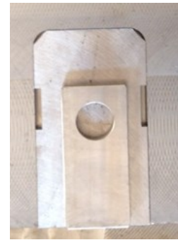
Two-piece safety plate (not welded)
