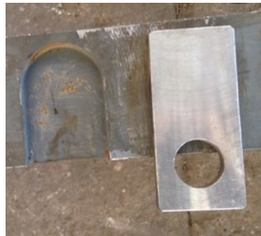
Upper part of the safety plate with milling in the rail foot
