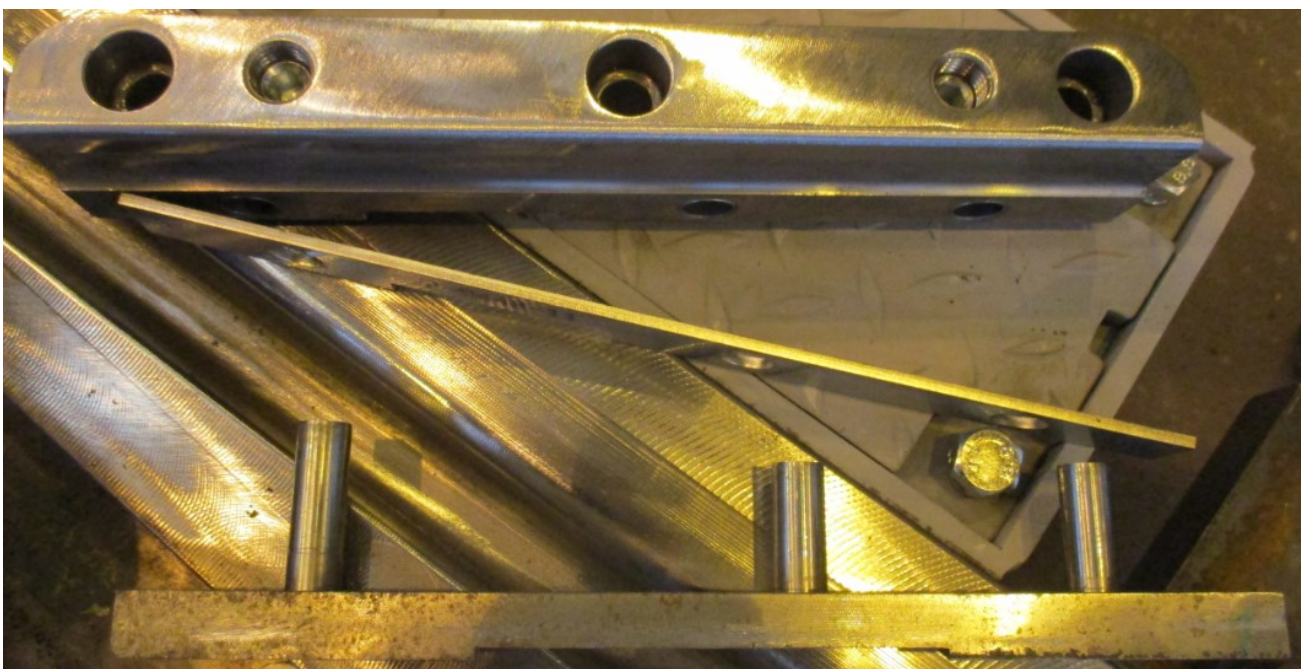
Disassemble the tongue clamp into individual parts, clean, visually inspect, lubricate the individual parts with a thin layer of copper paste- Cu7439 PLUS and reassemble.
