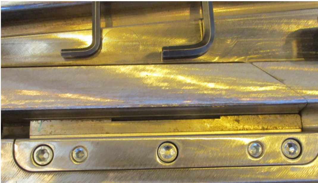
Use 2 Allen keys of the appropriate dimensions to remove the tongue clamp
