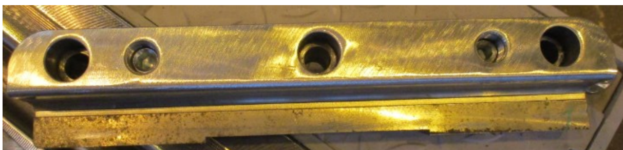
First clean the set of the tongue clamp all around
